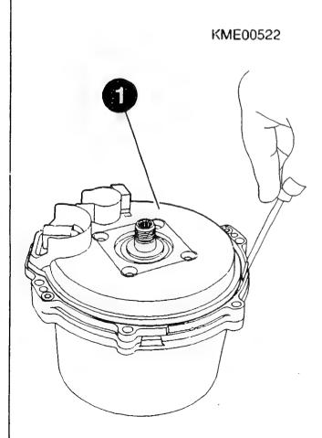
DISMANTLING AND CHECKING ALTERNATOR Dismantling cap Take out O-ring (1). NOTE: O-ring is always to be replaced.
